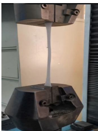
Figure 1. Tear strength test using a universal testing machine.
