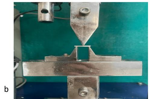
Figure 3: (a) schematic diagram of the three-point flexural strength test apparatus, (b) image of universal testing machine and testing bar.
