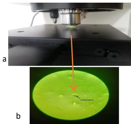
Figure 2: (a) Vickers micro-indentation testing machine, (b) image of indentation.
