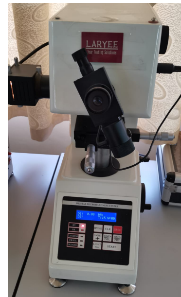
Figure 1. Vickers microhardness test.
