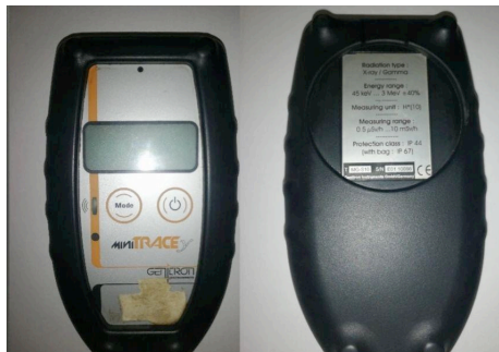
Figure 2. Radiation measuring device used in the study.
