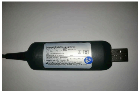
Figure 3. Intraoral digital sensor used in the study.
