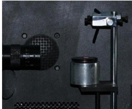
Fig. 1. Contact angle goniometer.
