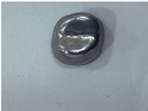
Figure 5. Titanium metal copy fabricated by CAD/CAM.
