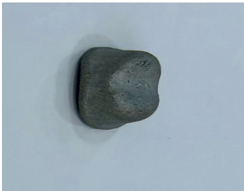
Figure 7. Metal copy fabricated by 3D printing.
