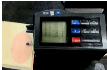
Figure 2. A profilometer instrument to measure the surface the roughness of specimen.
