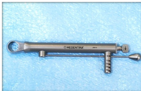
Figure 1. Manual calibrated torque ratchet with torque scale (10-70N/cm) (Medentika Co., Germany).
