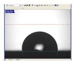
**Fig. 3.** Contact angle measurements shown on the software (SCA 20 DataPhysics, Germany)
