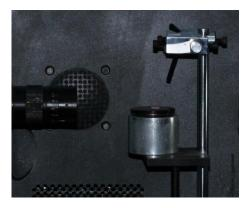
Fig. 1. Contact angle goniometer.
